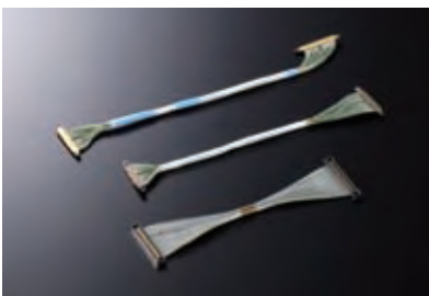
Micro Flex Coaxial (MFCX™) Cable MFCX™ cable has an extremely small outer diameter ranging from 0.20 to 0.35 mm. This cable is mainly used in the hinge connection area between the motherboard and LCD of a laptop PC or mobile-phone. Double-shielded structure is also available to enhance noise immunity.
