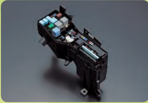
Compact, High-Reliability Relay Box By adopting the semiconductor relay and a new heatsink structure, we achieved miniaturization and weight reduction of our high-reliability relay box.
