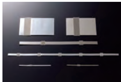
Tab-Lead Tab-Lead is used to draw electricity from lithium-ion batteries or electric double layer capacitors covered with aluminum laminated film. This wire is remarkably resistant to battery electrolyte. Also, its insulating layer prevents heat deformation. These characteristics provide excellent sealing reliability.
